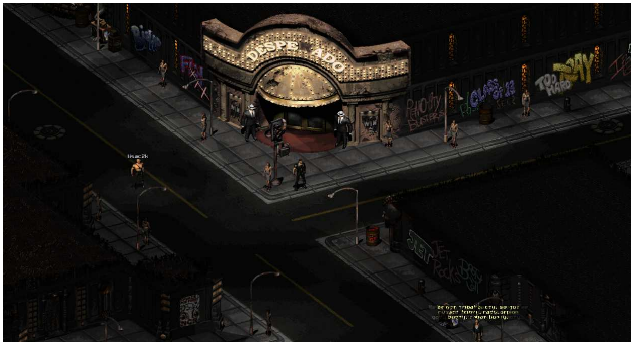
Illustration 9: Lighting emulated by adjusting lightness in 5 steps [0, -20, -40, -60, -80] for 5 light rays group. The lightness interval is [-100,+100], with 0 representing the neutral value.
