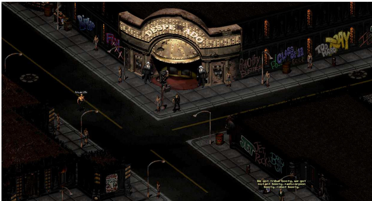
Illustration 8: Lighting emulated by adjusting brightness in 5 steps [-6, -12, -18, -24, -30] for 5 light rays/shafts groups. The brightness interval is [-100,+100], with 0 representing the neutral value.
